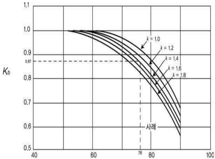
$$\text{게이지배압}(\%) = \frac{\text{배압}(\text{kPa}(\text{g}))}{\text{설정압력}(\text{kPa}(\text{g}))} \times 100$$
