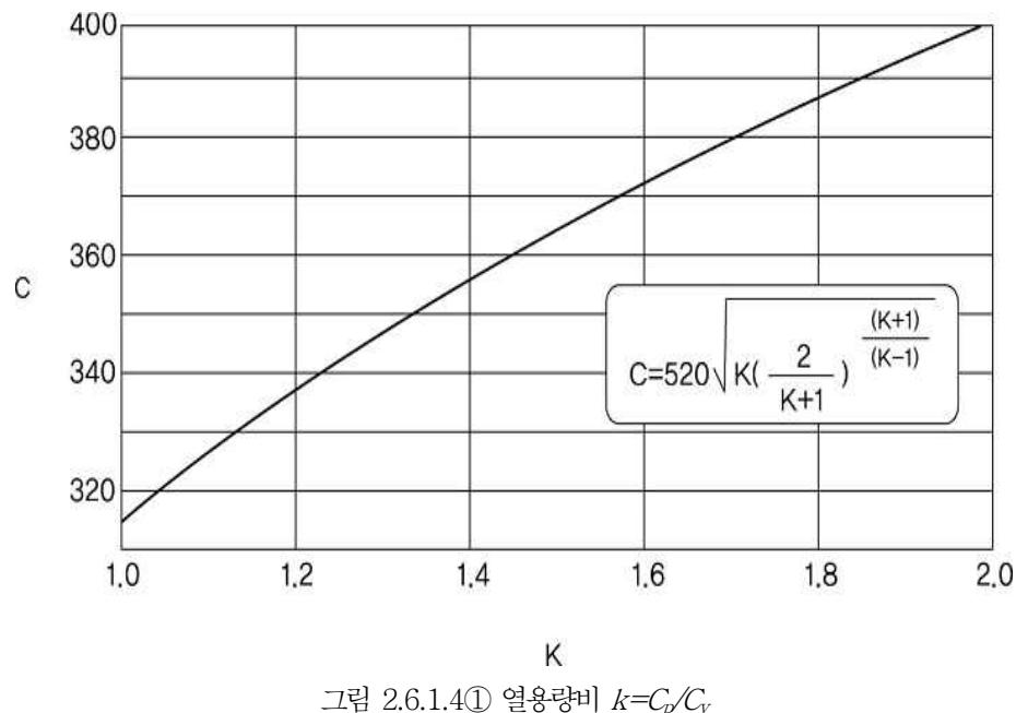
그림 2.6.1.4① 열용량비  $k = C_p/C_v$
