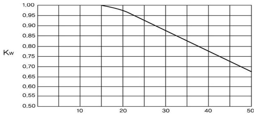
$$\text{게이지배압(\%)} = \frac{\text{배압(kPa(g))}}{\text{설정압력(kPa(g))}} \times 100$$
